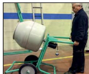
**CON MOTOR Y REDUCTOR PROVISTO DE DOBLE AISLAMIENTO TÉRMICO**
